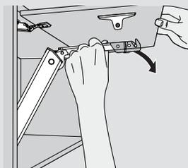
**C** Remove lift mechanism from door.
